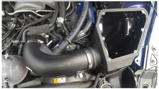
13) Attach remaining hose clamps and tighten, attach air filter and tighten clamp, screw bolt from stock air box to new air box to secure it in place, connect MAF sensor and holding clip to air box.
