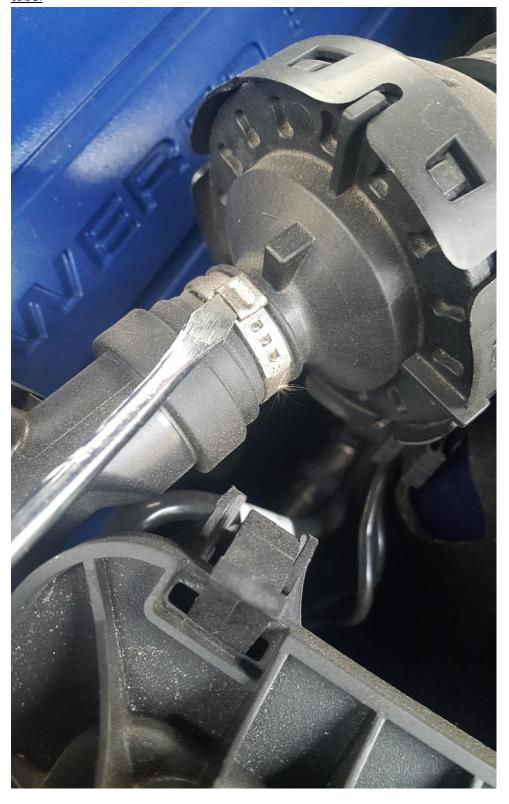
8) Remove the stock intake by wiggling it out from the throttle body and pulling it out from its location.
