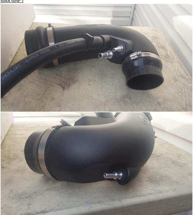
11) Insert MAF sensor into the new intake tube and tighten provided screws with an Allen key (\*Make sure the orientation is the same as it was on the old intake\*).
