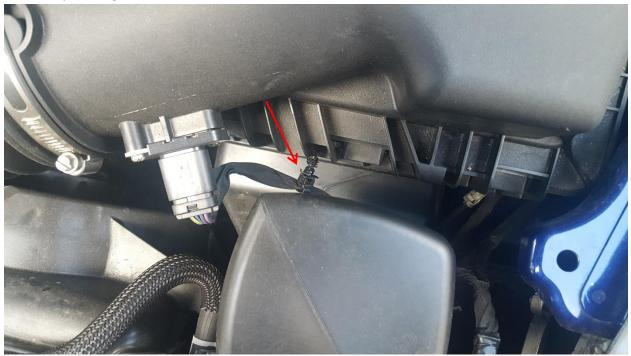
6) <u>Disconnect MAF sensor by pulling on red clip and using a star key unscrew the MAF sensor screws and gently remove the sensor (note the orientation of the sensor when inserting into new cold air intake).</u>
