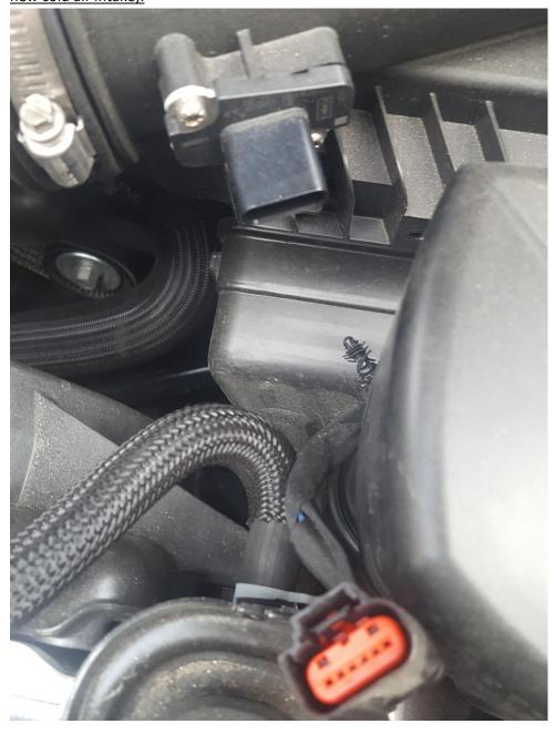
7) <u>Using a flathead screwdriver, remove clamp from other side of sound tube and remove the tube.</u>
