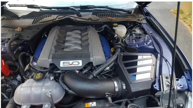
1) Begin by removing the engine cover, firmly pull at each corner until it pops out.
