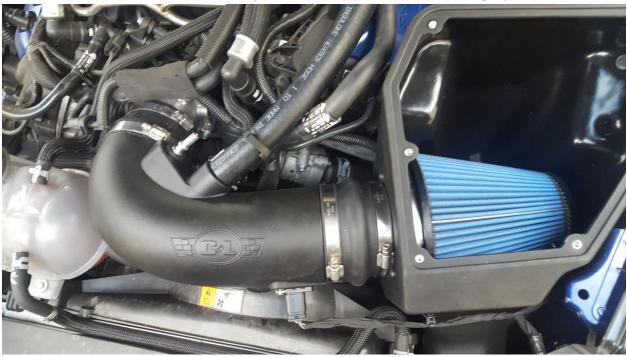
14) Connect all hoses to intake tube and connect air hose using speed clamps.
