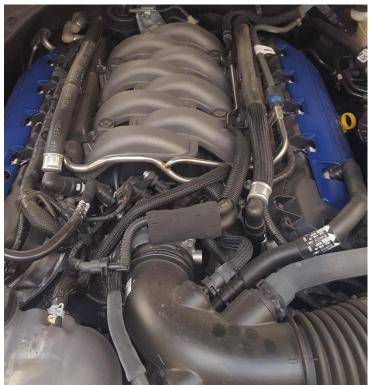
2) Remove stock air housing bolt with 10mm socket.
