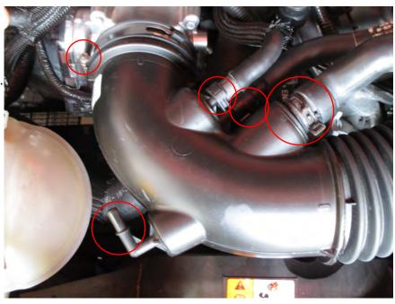
Step 3: Pushing the dark section of the hose clamp will allow you to pull the vacuum line off the intake tube.
