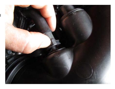
**Step 4**: Rotating the gray clip on the PCV hose will a pull the PCV line from the intake tube.
