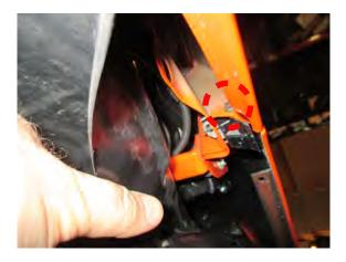
**Step 7:** With the splash shield removed, you can access the back plugs for the turn signals and fog lights.
