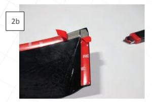
Peel the backing from the 3M tape. With help, begin to position spoiler over the rear window.
