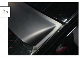
Line up the outside edge of the spoiler just inside the edge of the side and top of the glass. Once positioned apply firm even pressure over the length of the spoiler to ensure proper contact.
