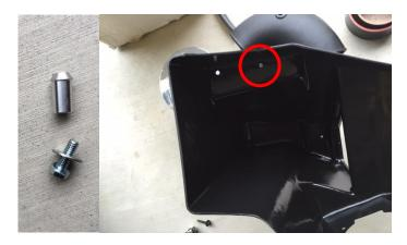
Step 9: Install the aluminum stud into the front hole Steeda air box. The assembly and location is pictured above. This will locate the Steeda air box into the grommet you just reinstalled in the fender.
