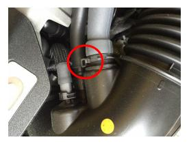
Step 3: Using a set of pliers, remove the factory sound tube from the intake tube. Circled above are the tabs you will need to compress together. There is a small tab integrated in the clamp that will hold it open after you compress it.
