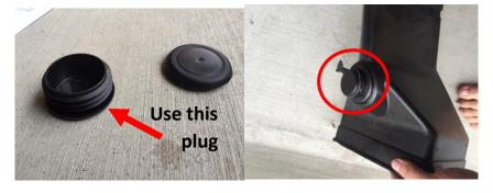
Step 17: Plug the hole left by the removed resonator as shown above. The assembly will then clip into place on the bottom of the Steeda air box over the three pre-adjusted screws on the lower opening of the air box.
