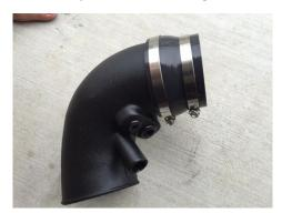
Step 20: flip the intake tube over and install the reducer coupling and supplied hose clamps on the smaller or throttle body end of the intake tube as shown above. You can now install the assembly on the throttle body.
