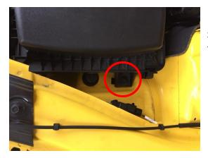
Step 6: Unbolt the lower portion of the air box from the fender using a 10mm socket and wrench.
