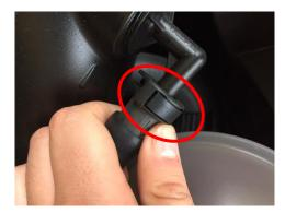
Step 4: Disconnect the remainder of the of the hoses attached to the intake tube. There are two that are accessible after removing the sound tube and one located on the bottom of the intake tube. Simply press the release button pictured above and pull to remove.
