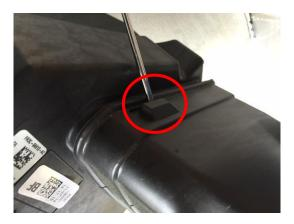
Step 15: Remove the lower inlet snorkel from the factory assembly to your Steeda assembly. The inlet is secured in three places on the factory assembly and can be popped from its place with a flat head screwdriver.
