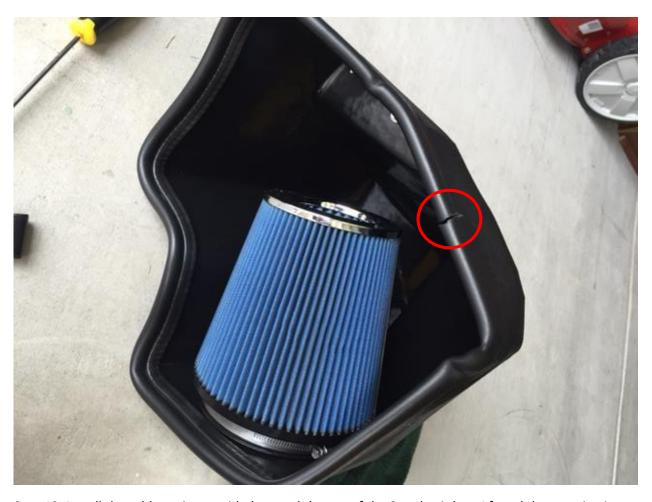
Step 13: Install the rubber trim provided around the top of the Steeda air box. I found that starting in the location circled above will hide the seam of both ends when installed in the car. You may need to trim away excess.
