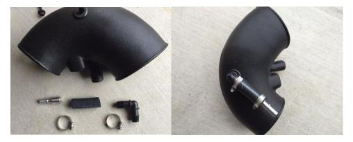
Step 19: Assemble the lower PVC adapter and install into the Steeda inlet tube as shown on the right. Place the aluminum adapter in one end of the hose and the plastic elbow in the other. Tighten both hose clamps and install facing the smaller diameter opening in the inlet tube. (throttle body end)
