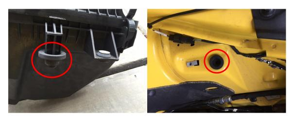
Step 8: Remove the rubber grommet from the bottom portion of the air box and reinstall it in the fender. (circled above)
