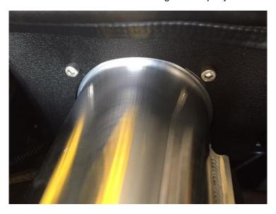
Step 10: Install the Aluminum velocity stack into the Steeda Air box. Pass the housing through the air box and orient it such that the opening for the MAF sensor will face the front of the car when installed. Complete using the four supplied ¼-20 bolts (7/16" head) and tighten them.
