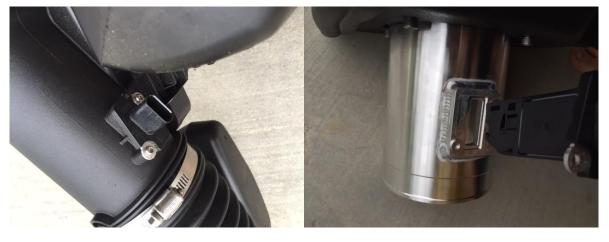
Step 14: Transfer the Mass Airflow Sensor (MAF) from your factory assembly to the Steeda assembly. Install the sensor with the black side up as pictured on the right. A T20 torx will be used to remove the MAF from the factory location and a T10 torx or 5/16" allen wrench will be used to secure the two new screws provided to install the MAF in the Steeda housing.
