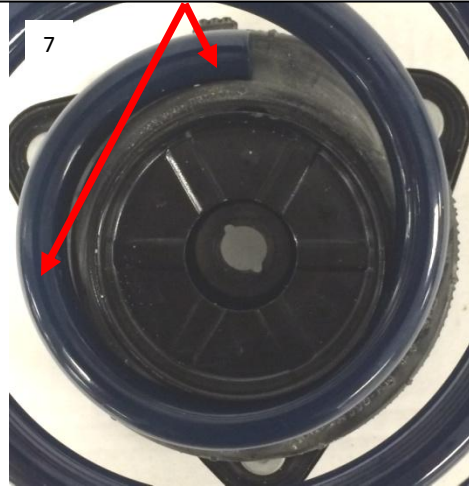
Incorrect , notice how the coil only wraps 1/4 of the way around the upper spring seat.
