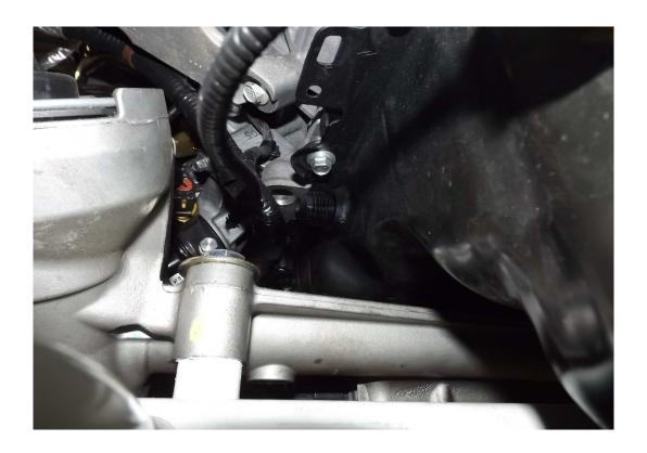
16. Now let's begin installing the turbo kit. We're going to start with the Y pipe that connects to both manifolds. You can also install both of the wastegates once the pipe is bolted in. I recommend leaving these bolts loose as to give you some adjustment when installing the next pipe.
