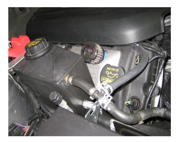
29. Install both valve cover breathers onto the engine. Use the supplied 5/8<sup>th</sup> caps on the intake manifold.
