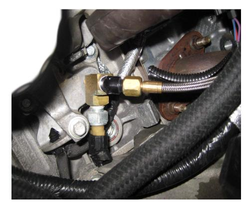
24. Install the oil feed line onto the turbocharger, using the supplied line, 90 degree fitting and adapter.
