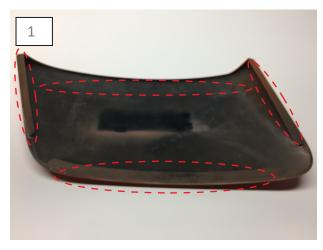
Clean the tape mounting surfaces with the supplied alcohol. Also, ensure the vehicle's paint is clean and free of dirt. Use the supplied alcohol wipes to clean the scoop mounting surfaces on the part and the car.
