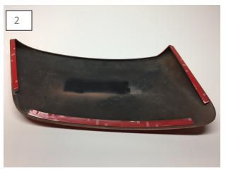
Apply the supplied adhesion promoter, allow the promoter to flash dry. then install the supplied tape to the scoops mounting locations.
