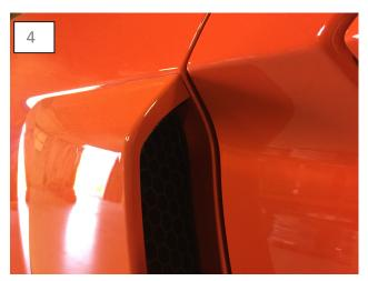
Test fit the part before removing tape backing. The top edge of the scoop sits slightly below the body line and slightly behind the door edge.
