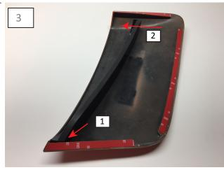
Next, install the supplied side scoop insert. Begin by testing fitting the insert. They can only be installed by inserting the bottom edge first and then sliding the top edge in second.
