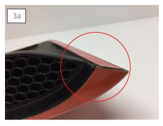
The insert has to be flush with the edges to ensure the scoop will fit correctly on the car. After you see how the insert fits, remove the tape backing and secure the insert to the side scoop.
