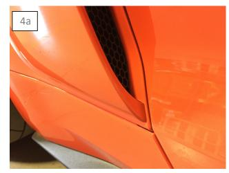
Line up the lower edge behind the door edge. Then remove the tape backing and apply firm pressure to the tape edges securing it to the car.
