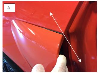
Begin be removing the side scoop from the vehicle. The side scoop can be difficult to remove. Use thick dental floss or fishing line, to "saw" the double sided tape. Pull the scoop off the car slightly to get the floss/fishing line between the scoop and the quarter panel. Pull the floss/fishing line side to side effectively cutting/sawing through the tape. \*\*Note: Trying to pry/pull the scoop off can damage the part and/or your vehicle.
