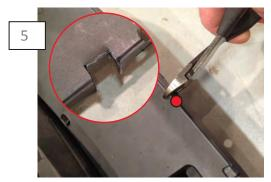
Some cars will require trimming of the splash shield in order for the clips to seat properly. A pair of wiring cutters will do the job. After drilling the appropriate holes through the chin spoiler. Mark the holes on the splash shield. Remove the splash shield (step6) from the car and trim a ¼" away from the outside diameter of the hole.
