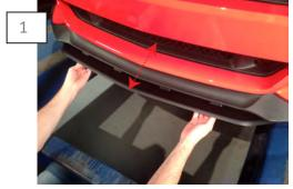
Raise and support the front of the vehicle. Center of the splitter with the center line of the bumper.
