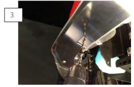
Have a helper hold the splitter while you drill the mounting holes in the chin spoiler. \*\*Note: Be very careful when drilling so that you **DO NOT** drill through the top side of the chin spoiler. Firmly press the supplied ¼" mounting push pins. \*\*Note: If you can not get the push pin all the way in you may need to trim the splash shield. See step 5 and 6.
