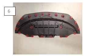
Removing the splash shield will require you to remove various clips, and 7mm screws.
