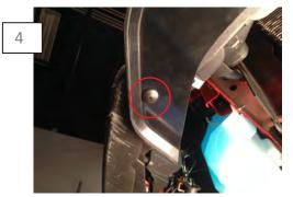
Optional: if you would like to tuck the side of the splitter tighter to the bottom of the chin spoiler, you will need to drill (2) additional holes. Locate a portion on the splitter that makes good contact with the underside of the chin spoiler and drill a  $\chi''$ hole through the splitter and the chin spoiler. Firmly press in the additional push pins as you did in step 3.
