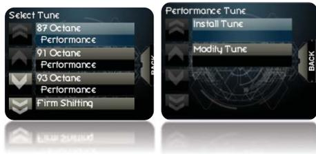
**Step 6:** The Trinity may prompt you to “turn your key on, but don’t start engine” and then ask you to turn the key on/off a few times. It will begin flashing your vehicle with the chosen tune. When the flash process is complete, the button and Trinity will reboot. **DRIVE YOUR VEHICLE WITH THE NEW TUNE!!!**
