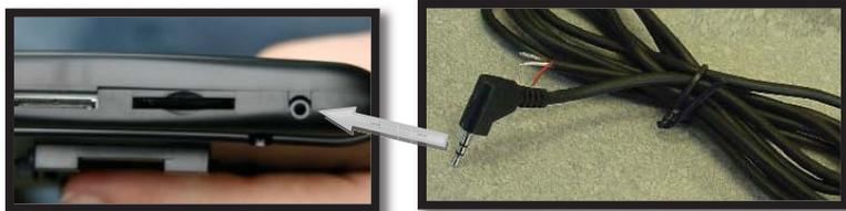
Example: Trinity Part # T1015 Analog I/O Cable available at [www.diablosport.com](http://www.diablosport.com). The T1015 is produced by DiabloSport to make hooking up external sensors much easier take a look at the following diagram to see which wire to use to connect your analog signal.
