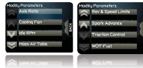
**Step 3:** To make changes to the parameter, use the touch screen on your Trinity and touch either the fine or coarse adjustment arrow (Fine adjustment is the single arrow, Coarse Adjustment is the double arrow). The numbers on the bottom right represent maximum parameter value
