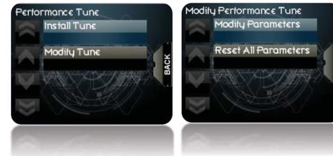
**Step 2:** Now you are in the “Modify Tune” Menu. You can scroll through the list of adjustable parameters by using the arrow icons on the left hand side of the screen, or alternatively with the buttons to the right of the Trinity’s screen. Choose the parameter you wish to modify and select it by touching it on the Trinity screen, or using the buttons on the Trinity and clicking the option with the center button.
