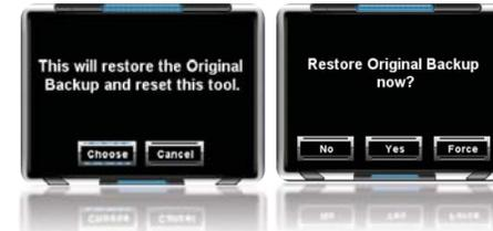
**Step 3:** The Trinity will begin writing the original backup to your vehicle and prompt you to turn the key on and off. After the flash process is complete, reboot the Trinity when prompted. Your Trinity will now be unlocked / unmarried from your vehicle and you can use it on a different vehicle, return to the dealership for service work, or bring it in for emissions testing!
