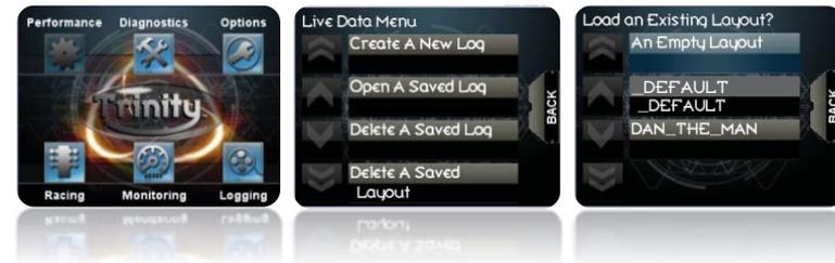
**Step 2:** You are now in the “Log Play/Record” menu and should see gauges present on the screen. Press the “RECORD” button on the right hand side of the Trinity screen, or use button 1. You can now choose if you would like to monitor real time data, or record the data you are viewing. Select “Record a New Log” and drive your vehicle.
