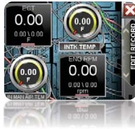
**Note:** You must have at LEAST 1 other OBD-II Parameter included in a NEW gauge layout in order for the analog input to function properly. This gauge can be included on the same page or on another gauge page.
