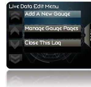
**Step 4:** To choose a gauge type, simply touch the gauge type you want to add (for more information on gauge types see section 2.1) to scroll through the different gauge types tap the arrow icons on the left side of the screen or use the arrow buttons to the right of the Trinity screen. For the purposes of this demonstration, let's select a large radial and then the parameter you wish to view (Engine Speed or RPM).
