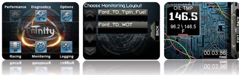
**Step 2:** Drive your vehicle and view the virtual gauges in real time. Many DiabloSport setups will have more than one "Gauge Page" or bank of virtual gauges. You can switch between different gauge pages on the fly by touching the screen or using the up and down buttons to the right of your Trinity screen.
