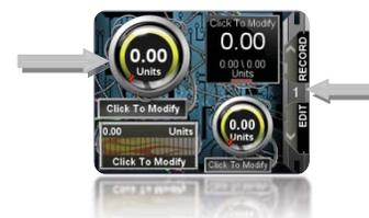
Other buttons on the right hand side of the screen will access addition menu options for the current mode the Trinity is in. This can be anything from edit, record, modify, or back.
