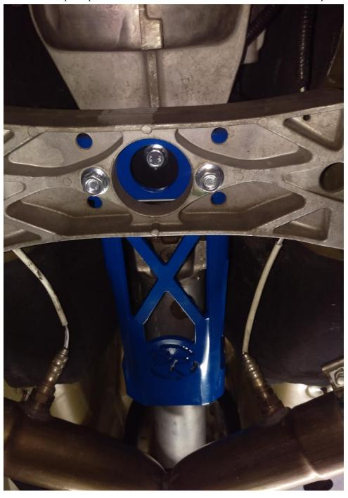
12. Reattach the crossmember to the car with the 4 factory bolts (Circled red below) and torque to 85 ftlbs.
