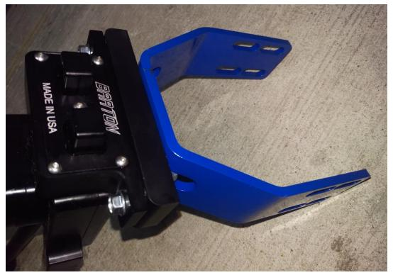
3. Install the upper half of the shifter bracket: Rotate the U shaped upper half of the shifter bracket up over the driveshaft. Attach the shifter mount to the U bracket using 2 x M6 bolts and torque to 6ftlbs.
