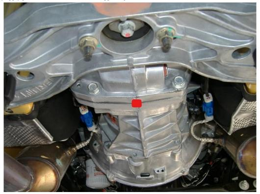
6. Remove the transmission cross member bolts (Circled red below) that hold the crossmember to the car.
