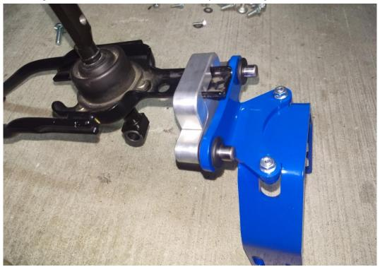
For aftermarket shifters, attach the bracket to the new appropriate adapter with provided bolts. Torque the bolts to 6ftlbs.
