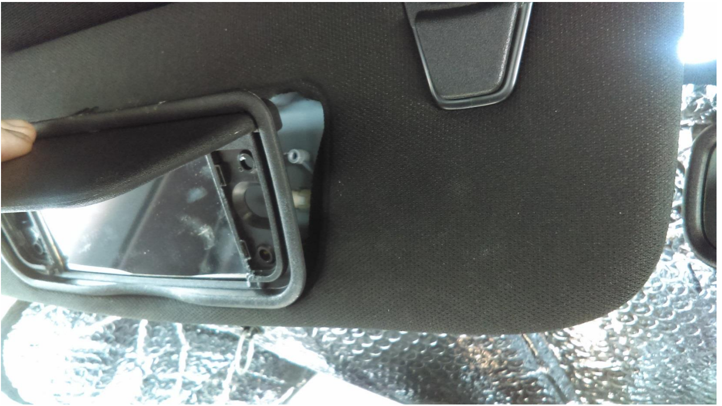
Step 4: Replace bulb and re-install in reverse order of removal. Repeat process on passenger side.
