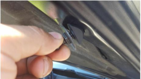
4.) Use a 14mm deep socket to tighten the mounts to the hood.
