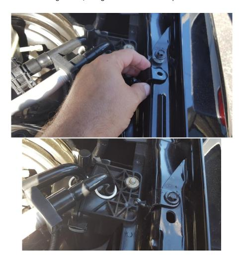
7.) Install the Gas Strut on the upper bracket, then the lower bracket.
