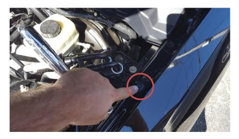
6.) Install the fender mounting bracket, facing down as shown in the picture.
