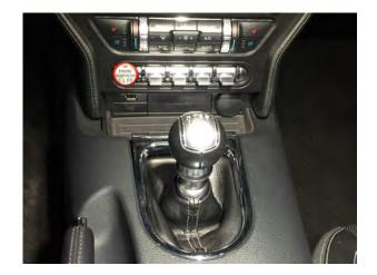
Remove the factory shift knob by rotating it counter clockwise.
