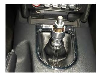
Install the supplied nut. This nut is used to align the shift pattern on the shift knob. Thread the shift knob on until it is tight against the nut. If the shift pattern does not line-up simply adjust the nut up or down until it does. \*\*Note: Ensure the reverse lockout is still functional. If not, loosen the lock nut and knob until it does.
