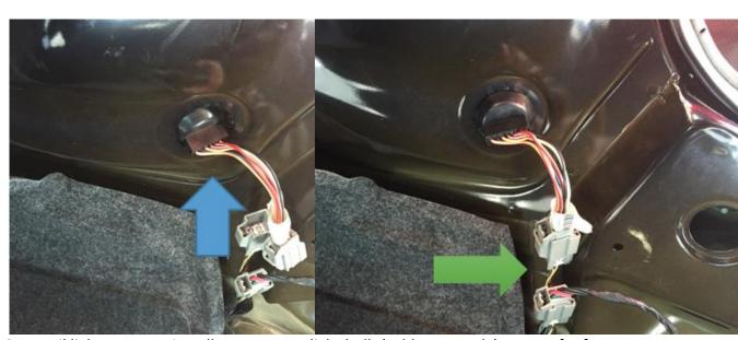
**9.** Once tail lights are out, install new reverse light bulb (sold seperately) or transfer from previous tail lights. To transfer, twist reverse light bulb harness until release. Hand pull bulb out from socket. Install in new Vector tail lights.
