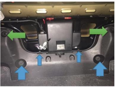
3. Take the slotted screw driver and pry out the FOUR plastic clips.
