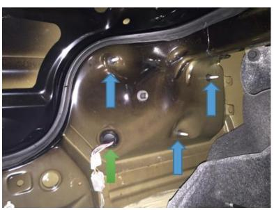
7. Take an 11mm deep socket and remove the nuts on all three bolts
