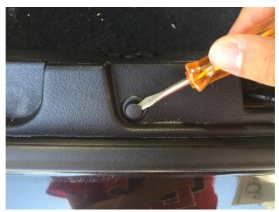
**4.** With your hand, unscrew the top TWO screws on both sides.
