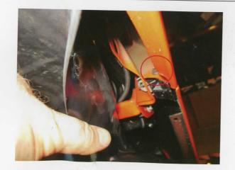
Fold back the fender liner so that you can access the one bolt that holds the bumper to the fender. \*\*Note: This bolt is tricky, it may help to remove the wheel for better access.
