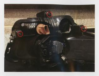
**Step 8**Remove the (3) 7mm screws holding the turn signal to the bracket. Then remove the turn signal.
