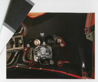
**Step 7**Using a 7mm socket, remove the screws holding the turn signal bracket to the bumper. Then gently pry the bracket from the bumper.
