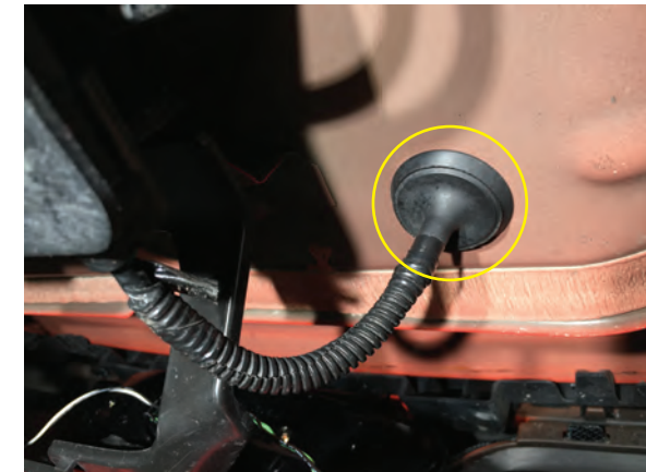
Step 4 Locate the body grommet on the bottom of the trunk. Carefully pierce only the body grommet so that you can feed the black and green wires from the reverse light into the trunk.
