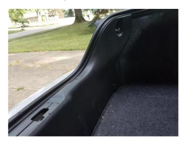
2. Remove rear plastic shield by pulling up and towards the cabin. Be sure not to damage the clips.
