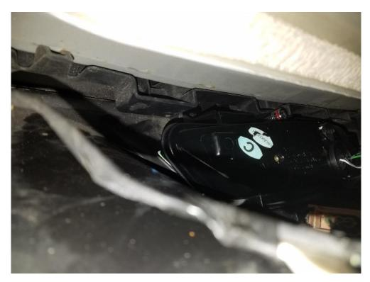
9. Secure the wiring plug so that it does not hang down, and rout the black and green wires up through the grommet shared with the spare tire pit. Use a screwdriver or knife to penetrate the grommet.
