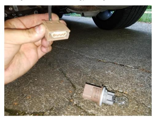
8. Install the replacement light fixture using the stock screws and your extended socket wrench. I found this to be extremely tricky and will require multiple tries. Be sure not to lose the screws. I used a socket to prop up the plastic part that gets in the way of the top screw mount locations.
