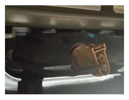
6. Here is a picture of the light removed. It is easier to see the locations of the 7mm plastic screws. DO NOT LOSE THESE, the replacement kit does not provide replacement hardware.
