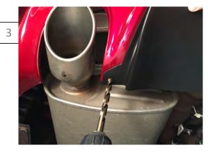
Drill a 23/64" holes through the bumper to secure the diffuser using the nylon push pin. Push pin fit very tight. \*\*Note: You may need to jack the rear of the car up to have enough space for the drill.
