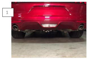
Ensure the rear valance is washed and free of dirt. Wipe the tape contact points on the bumper with the supplied alcohol wipe, followed by the supplied adhesion promoter. \*\*Note: A clean surface is essential for proper adhesion.
