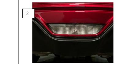
With the backing tape still installed, center the diffuser on the rear bumper. Line up the lower diffuser mounting tabs. Mark the center of each mounting hole.
