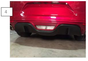
Remove backing tape and press in nylon push pins. Lay diffuser onto paint, carefully lining everything up with the reverse light. Apply firm even pressure on all tape ledges to ensure proper adhesion.
