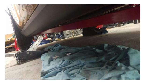
6. Using a marker, trace all weld surfaces then remove sub frame connectors.
