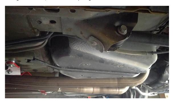
3. Using the same socket, remove the plastic fuel line cover on the driver's side.
