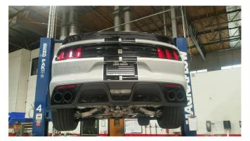
**Step 8.** Once a final position has been chosen for the new exhaust system, evenly tighten all clamps from front to rear using the torque specifications on page one of the instructions. Inspect all fasteners after 25-50 miles of operation and re-tighten if necessary.
