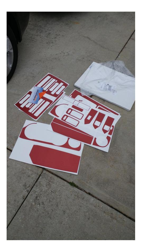
3. Peel each piece off of the sheets slowly. Spray each piece with the soap & water mixture liberally, not dripping, so that they do not stick to the surface immediately and will be easier to adjust if necessary.
