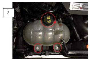
Remove the (2) 10mm bolts holding the coolant reservoir to the fan shroud.
