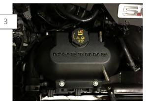
Remove the coolant cap, install the reservoir cover. Re-install coolant cap.
