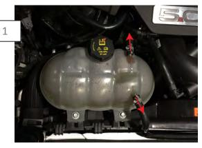
Using a pair of plyers, remove the (2) hoses connected to the coolant tank. \*\*Note: Some coolant will leak up, have some paper towels on hand.
