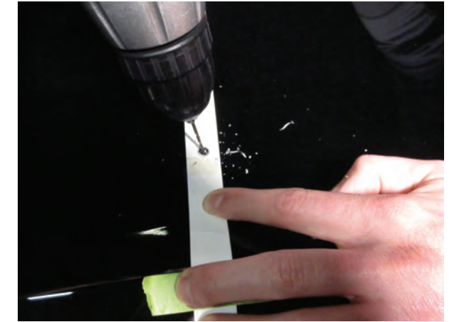
Step 7\\ Take the necessary steps to prevent metal shavings from scratching the paint, also prevent metal shavings from getting all over the engine bay using a drop cloth. Mark and drill a pilot hole on each of the (5) mounting locations. Once the pilot hole is drilled, drill a 9/32" hole through both the upper, and structural skins of the hood. **Note: Be careful not to drill past the structural layer as you may drill into important engine components.
