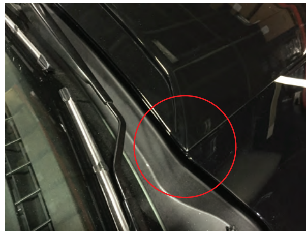
Step 4\\ Place the hood scoop on the vehicle, line the back edge of the scoop up with the back edge of the hood. Then center the hood scoop side to side.
