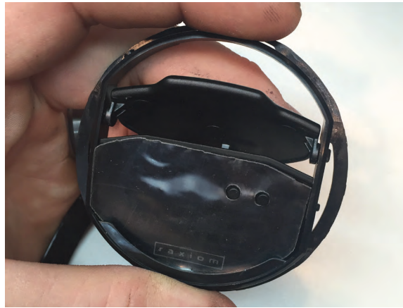
Step 8 Install the display into vent slat bracket. NOTE: Display glass goes behind lip at bottom of bracket.
