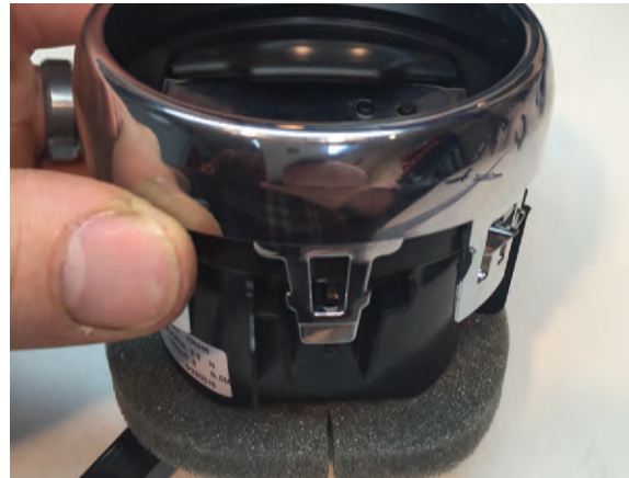
Step 11 Reinstall the chrome trim ring. **Note: The chrome ring can only be installed in one position. The tab with the two bumps lines up with the flat portion of the barrel.
