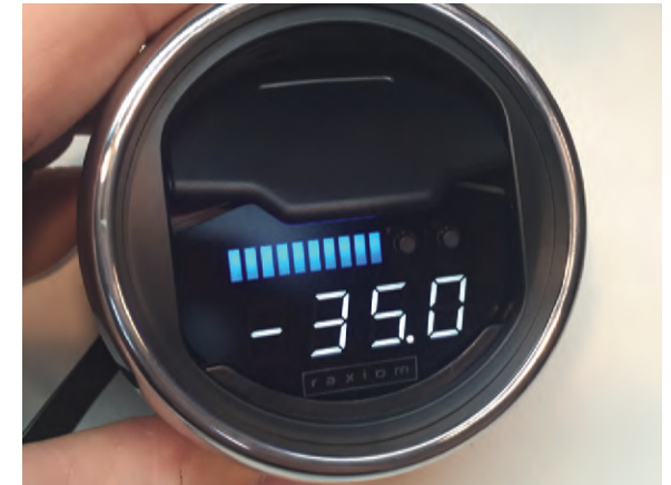
Step 12 Your gauge is now ready to be installed in your vehicle. **Note: Flat part of vent barrel is in the 6 o'clock position when installed in vehicle.
