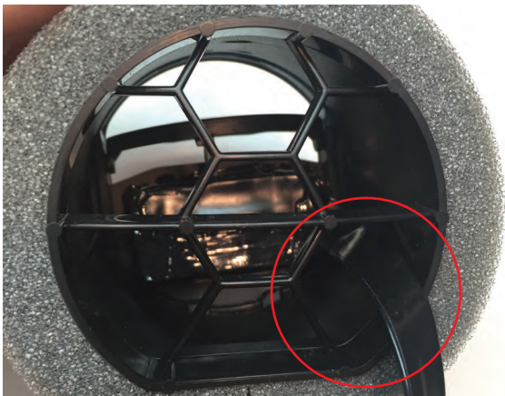
Step 10 When feeding the display cable through the back of the vent, make sure the cable goes through this hole.
