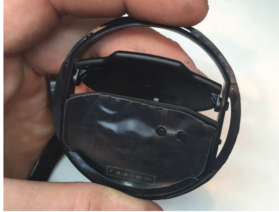
Step 8 Install display into the vent slat bracket. **Note: Display glass goes behind lip at bottom of bracket.
