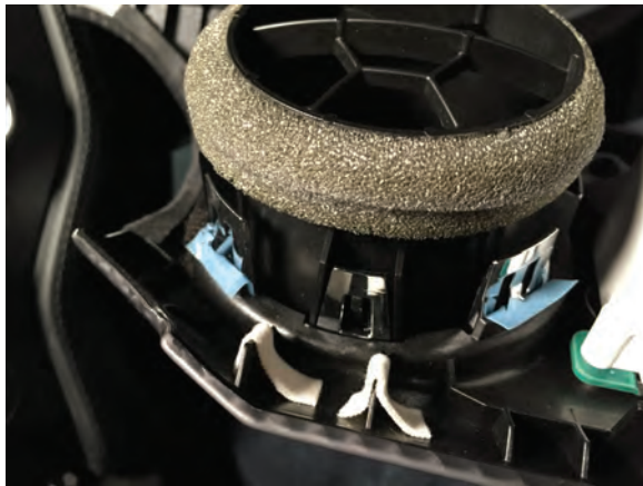
Step 4 Flip the dash panel over so you can access the back of the vent. Depress the chrome clips around the vent and push the vent through the front of the panel.
