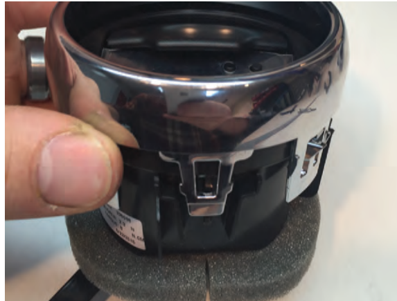
Step 11 Reinstall the chrome trim ring. **Note: The chrome ring can only be installed in one position. The tab with the two bumps lines up with the flat portion of the barrel.
