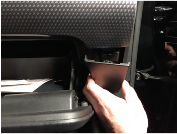
Step 1 Open glove box and remove the lower right hand trim panel. It is held in with plastic clips, rock the panel back and forth while pulling the panel straight off.
