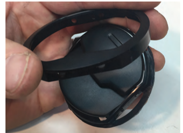
Step 6 Take the vent slat bracket out of barrel and remove black trim ring.
