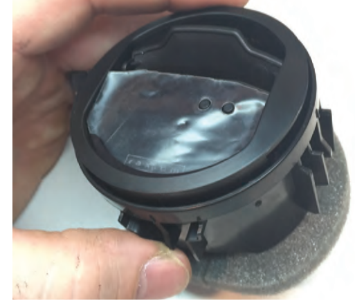
Step 9 Snap the black trim ring onto the bracket and install into vent barrel.
