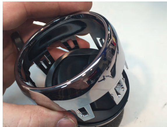
Step 5 Remove the silver trim ring from the vent barrel.
