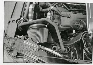
15. Install the K&N® air filter onto the adapter and secure with the provided hose clamp then secure the heat shield to the air filter housing mounting location using the provided hardware.
