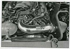
20. Install the K&N® intake tube into the hose at the filter adapter and then into the hose at the throttle body, adjust the tube and hoses for best fit and then secure with the provided hose clamps.
