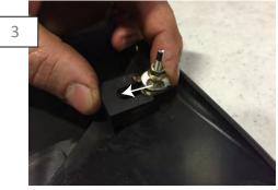
Install the supplied clip stud to the underside of the Hood Vent Scoop.
