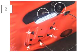
Remove the (2) 9mm nuts holding the factory vent in place, depress the vent clips on the underside and remove.
