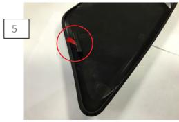
Test fit the Vent Scoop. Then remove the 3M tape backing from the mounting lip.
