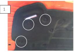
Remove the hood liner push pins and hold back the liner to gain access to the factory hood vent mounting nuts.
