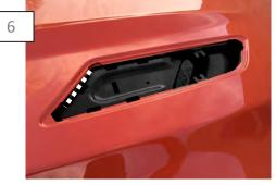
Apply downward pressure on the rear of the Vent so that the lip slides under the edge of the hood, then secure with the supplied washers and nuts.
