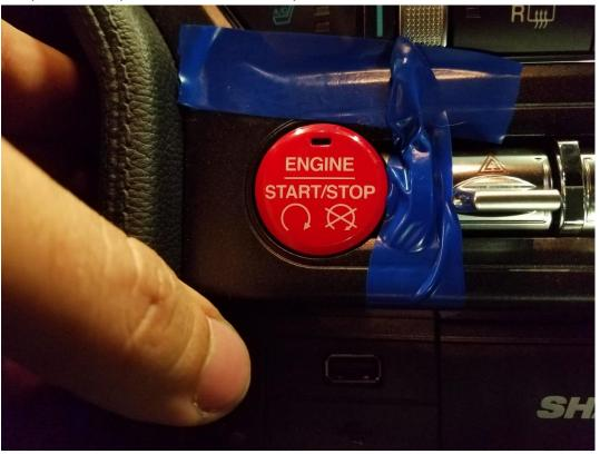
**5.** Remove tape from the center console and reconnect the battery. Test the switch to ensure the light still works and engine starts.
