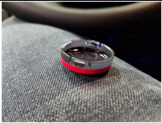
**4.** Line up the new switch with the led on the body and then firmly press in the middle so the snaps click into place on the switch body.
