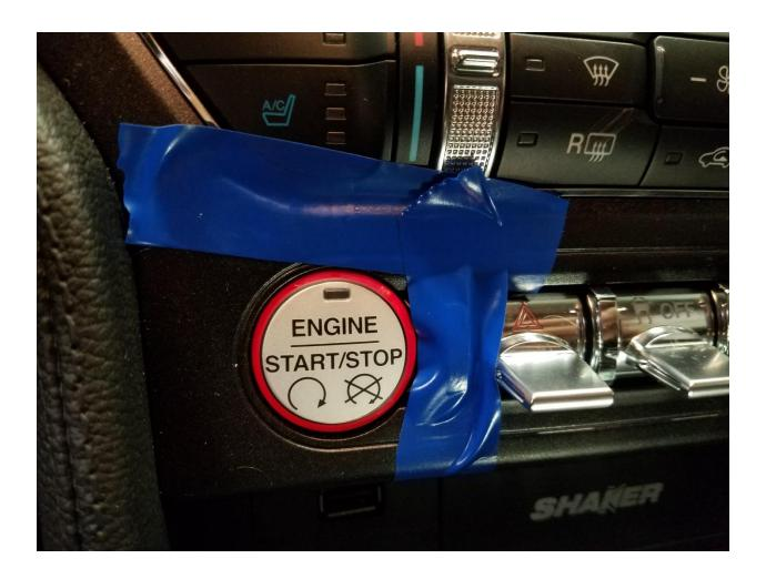
**3.** Now take the pick and begin to pry from the upper right corner (about 1-2 o' clock) on the switch. There is two retaining tabs at about 11 o' clock and 5 o' clock that you are attempting to get to pop off of the switch body. Take your time and do not rush as to not accidently scratch anything. Eventually the switch will pop off.
