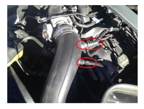
5. Remove the clamps with an 8mm socket or Flathead screw drive. Remove the Intake tube and set aside
