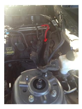
**13.** Remove the pin type harness holder located near back of the Intake Manifold.
