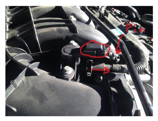
**12.** Move the Injector Insolating Foam out of the way an up the fuel line... It's quite Dusty!
