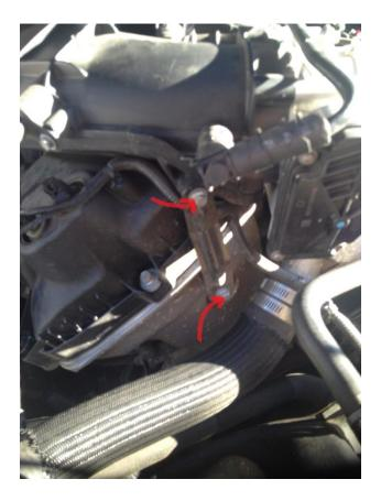
**10.** A Pinch the Brake Booster Hose Clamp off with Pliers (Circled in red) and disconnect the lines. Then remove EGR Hose from its Holder (Red Arrow)
