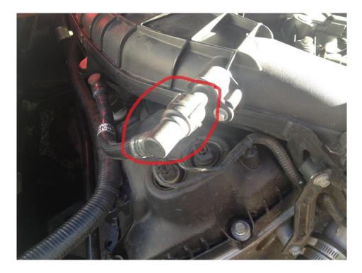
9. Remove the Intake support bracket by removing the (2) 8mm bolts. Set aside
