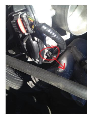
8. Remove the Passenger side PVC tube quick disconnect
