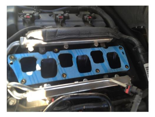
**17.** Place the spacer on top of gasket in the correct orientation and align with gasket.
