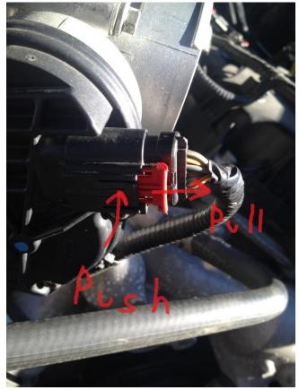
7. Then remove the plastic pin harness holder from its location
