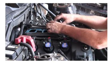
11. Put the upper plenum back in place with the existing hardware still in the manifold holes.
