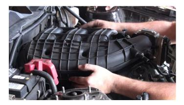
12. Tighten the 7 bolts until snug to ensure a perfect seal. Place close attention not to over tighten.
