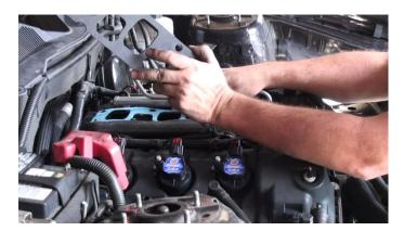
10. Place the .400" plenum spacer on top of the gasket and again ensure the patterns line up.
