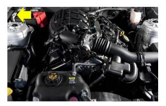
3. Remove the wiring harness that connects to the Mass Airflow Sensor.
