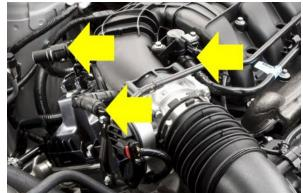
8. Unbolt the 7 bolts outlined in the photo below but DO NOT remove. Simply unscrew them completely and lift off the upper plenum.
