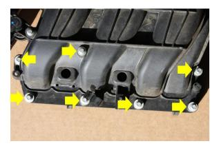
9. Your upper plenum has an O-ring style seal that is reusable. Place the supplied gasket on of the lower manifold, ensuring the patterns match up.
