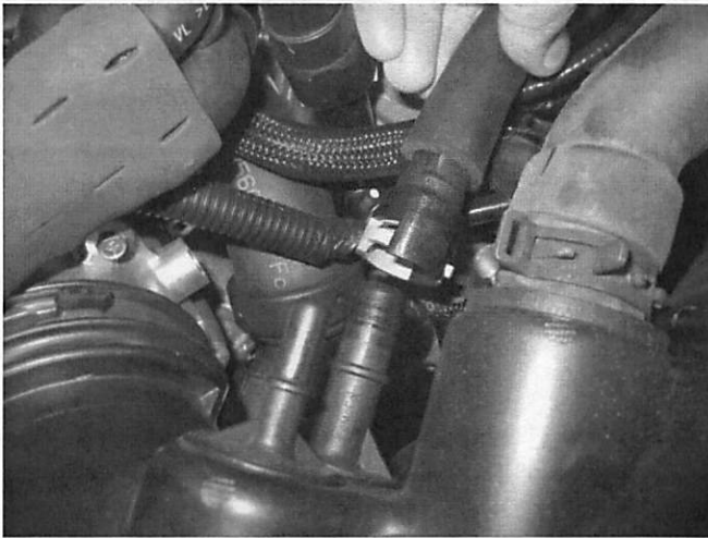
5. Disconnect the crankcase vent hose from the factory air duct.
