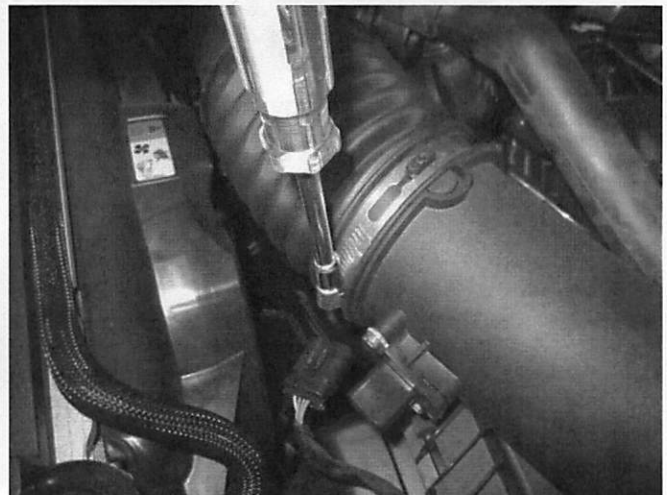
8. Loosen the clamp holding the factory air duct to the air box.
