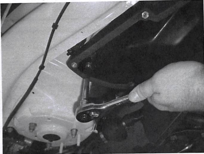
14. Tighten the air box in place using the factory 10mm bolt.
