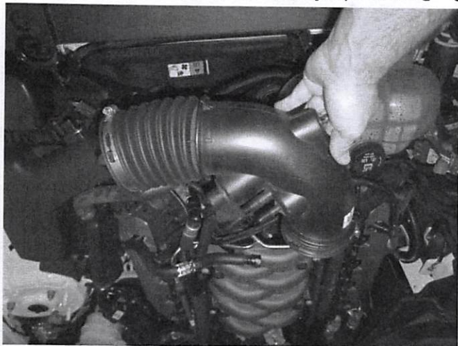
9. Remove the factory air duct from the engine compartment.
