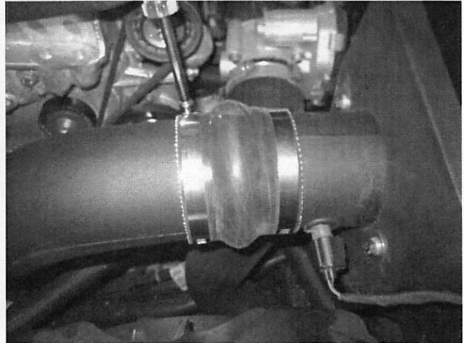
18. Tighten the CORSA duct onto the filter adapter using the 3.5in hump hose with the supplied #56 clamps using a 5/16 socket or nut driver only.
