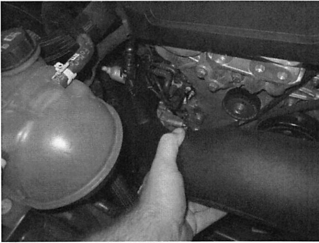
17. Slide the CORSA duct into the reducer but do not tighten the clamp at this time.
