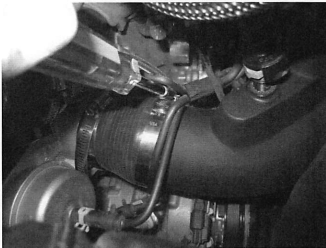
19. Tighten the reducer to the CORSA duct with the #48 clamp using a 5/16 socket or nut driver only.
