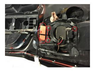
**Step 8** Install the replacement lights, and mount the control box to the fog light bracket as seen above.
