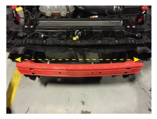
**Step 9** Feed the wiring harness extension behind the crash bar along the factory wiring harness. The pigtails of the wiring harness will end up on the driver side.
