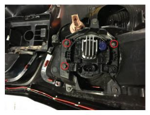
**Step 7** Using a 7mm socket remove the factory fog lights.
