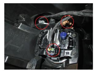
**Step 6** With the splash shield pulled back, you can access the plugs for the turn signals and fog lights.
