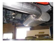
4. Once you have entire system hanging loose re install the factory fram support bracket. Instal the forward bolt loosly and used the supplied spacers and bolts for the rear 6 bolts. Tighten down all the bolts.
