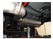
3. Now install the passenger side muffler assembly #B by sliding the metal hangers into the rubber grommets. Then do the same for the driver side muffler assembly #A. Use clamp #D to secure together. Keep loose.
