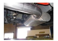
4. Once you have entire system hanging loose re install the factory fram support bracket. Instal the forward bolt loosly and used the supplied spacers and bolts for the rear 6 bolts. Tighten down all the bolts.
