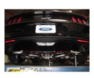
5. Check for clearance on all pipes and tip location. Place rubber objects or wood objects in areas that have little clearance. This will help hold the exhaust in place when you begin to tighten everything down. Once you have everything in place, firmly tighten all bolts and clamps down securely. Remove objects holding parts in place and double check all clearances.
