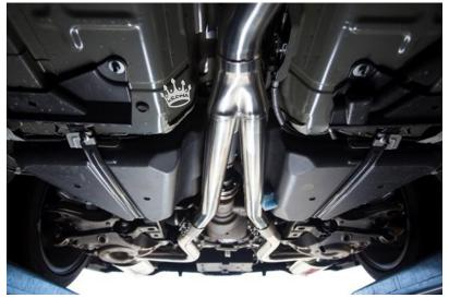
9. Tighten down the 2.5" compression clamps and then the 3" band clamp on the mid pipe section. See below for proper clamp orientation.
