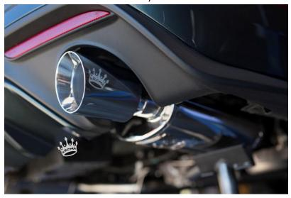
8. When tightening down all bolts and clamps working your way forward it is important to also ensure all piping in parallel to the ground. This indicates proper fitment has been achieved.
