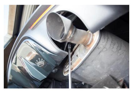
4. Next you may remove the factory rear exhaust hangers holding the system to the rear suspension just above the differential cover(x1 13mm bolt each side). These hangers can remain on the system until it is removed from the vehicle. Spray some lubricant on the rubber portions as you will need to remove these and reinstall on your new Krona system.
