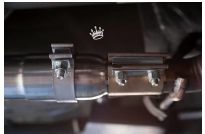
10. Double check all your connections, bolts and tip section placement. Final assembly should look as shown below.
