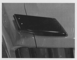
Step 5: Firmly attach the upper spoiler to the legs using the supplied M6 bolts and washers.
