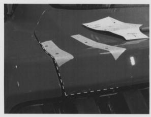
Step 2: Drill a pilot hole then finish with a 21/64" diameter hole.
