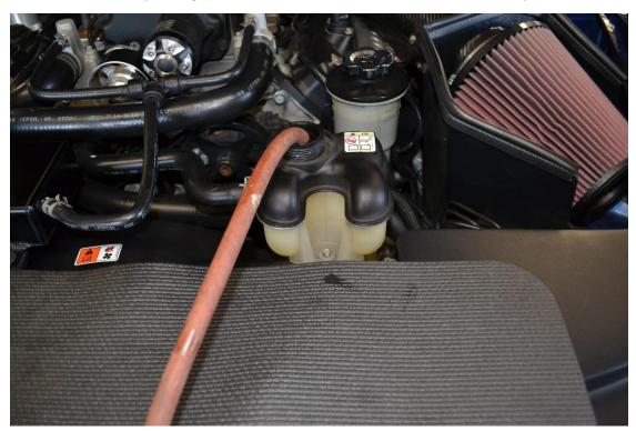
b) Use a set of pliers and loosen the clamp, remove line from tank and allow the fluid to go in a drain bucket or pan.
