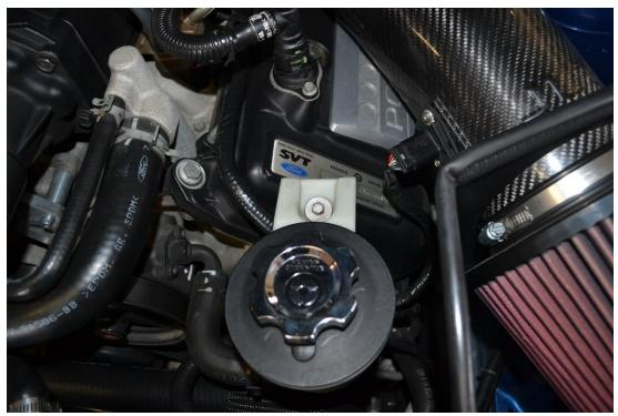
27. Use a set of pliers to loosen the hose clamps that attach the fluid lines to the reservoir, remove each hose from the tank and remove stock tank from vehicle
