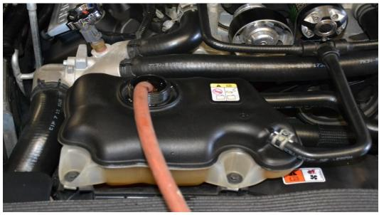
a) Using a 3-4 feet of hose (or siphon kit) to siphon the coolant out of the tank into a bucket. Siphoning the coolant makes it the cleanest and easiest way to remove it from the tank.
