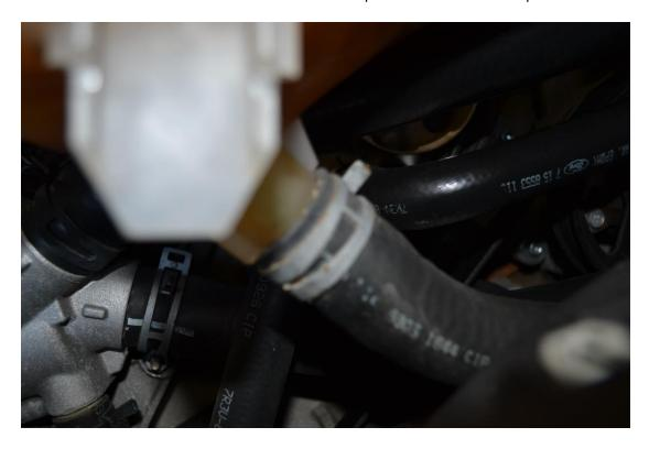
8. Once the line is removed from the tank, make sure the line is aimed upwards so the coolant in the line does not pour out. If the hose is full to the edge, dump some of the excess fluid into a cup. Then you might be able to use another hose to keep it upright
