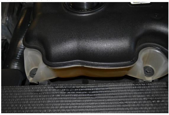
7. Once bolts are removed, lift the tank off the vehicle enough to remove the coolant line attached to the bottom of the tank. You would need to use pliers to loosen the clamp to remove the line.
