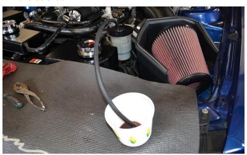
26. Use a Ratchet and an 8MM Socket to remove the bolt from the back of the reservoir which holds the reservoir to a bracket.
