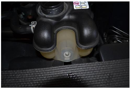
17. Use a set of pliers to loosen the hose clamps that attach the coolant lines to the tank, remove each hose from the tank and remove stock tank from vehicle.
