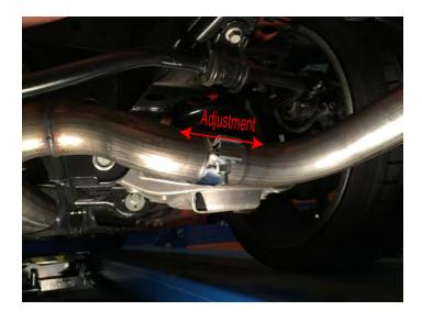
**Step 4:** Mount the muffler bracket to the chassis using the factory hardware.
