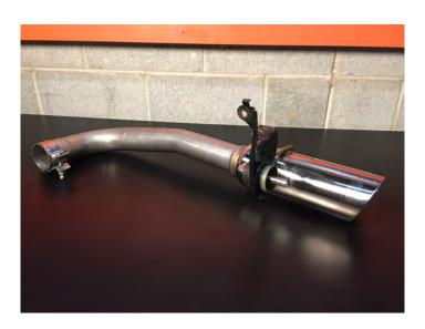
**Step 3:** Install the muffler delete, slide the delete on to the exhaust. Do not tighten the clamp yet. See Step 5.
