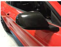
Thoroughly clean the vehicle's paint/plastic ensuring it is wax and grease free. Then peel the tape backing off and install.
