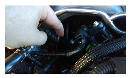
**Step 4:** Install your NEW JLT3.0 Oil Separator (supplied with factory connections for plug and play install)
