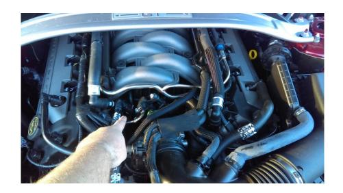
**Step 3:** Press down on grey clip and release the connector
