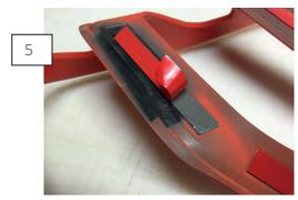
Remove the tape backing. Position the trim, and apply firm pressure to ensure proper adhesion.
