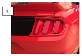
Test fit the trim panel on the tail light prior to removing the tape backing.
