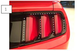
Begin by cleaning the tail light of dirt and debris using soap and water. Once thoroughly dry, wipe highlighted locations down the with the supplied alcohol wipes.
