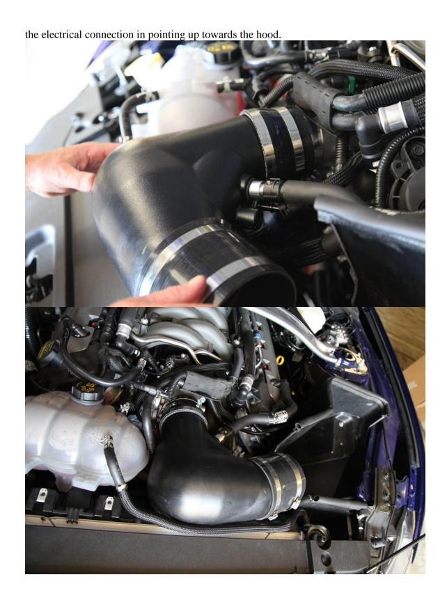
19: This step in very important. Make sure that throttle body coupling is pressed firmly and completely onto throttle body. If done correctly the large intake elbow will be touching the top of the fan shroud (see picture) this will ensure proper hood clearance.
