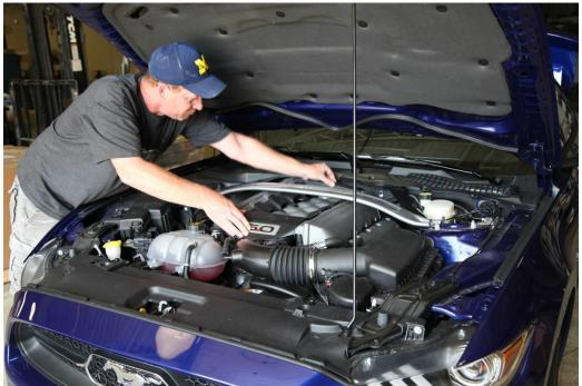
2: Disconect Mass airflow sensor connector
