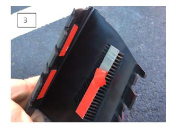
Remove the tape backing and apply the adhesion promoter. Allow the adhesion promoter to flash dry. Then position the grille extensions.
