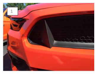
Begin by test fitting the extensions. \*\*Note: which extension goes on which side.
