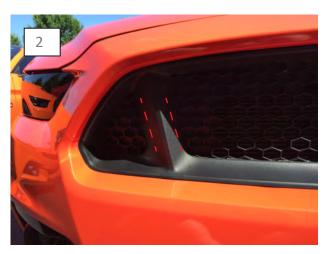
Clean the grille of dirt and debris using soap and water. Once thoroughly dry, wipe the highlighted locations down the with the supplied alcohol wipes.
