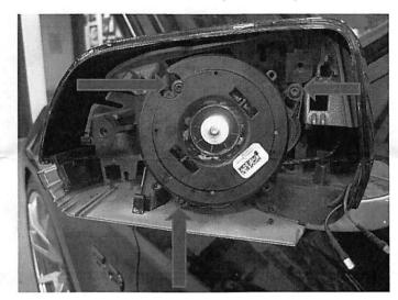
6. Disconnect connector as shown below, and set adjuster aside.
