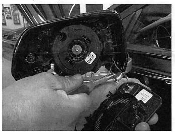
3. Remove the (2) T-15 screws that secure the outer ring to the mirror housing. Use small Screwdriver to release clips, and remove outer ring.
