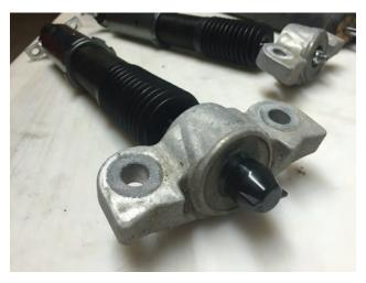
**Step 13:**Lengthen the shock body by unscrewing the lower shock mount until the shock is long enough to bolt on. Install the shock.
