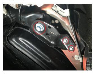
**Step 5:**Locate and remove the (2) rear-most rear subframe bolts.
