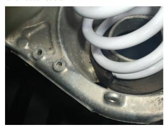
**Step 10:**Raise the rear subframe with the jack and slowly tighten the (4) rear subframe bolts. Then re-tighten the (4) front subframe brace bolts.
