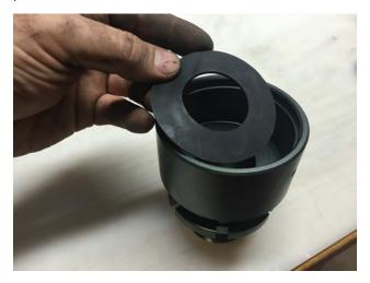
**Step 8:** Install the upper spring perch, use the set screw to hold the perch in place.
