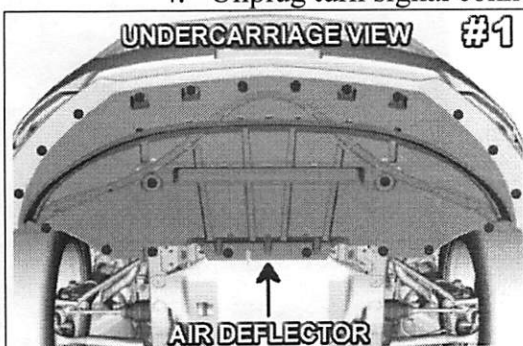
Remove air deflector. It is held by 16 screws/ 6 push pins (shown as dots).
