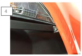
Before removing the tape test if the part so you can see how it fits the bumper. Apply slight pressure to the fog/turn signal bracket so that you can slide the bumper splitter between the bracket and the bumper.
