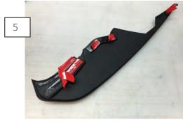
Once comfortable with the way the part fits, remove the tape backing. Apply the supplied adhesion promoter to the tape and allow it to flash dry. Then install the splitter to the bumper. Slide the splitter between the bracket and the bumper. Then apply firm even pressure to the velcro to ensure proper adhesion. Then Reinstall the bracket screw and fender liner.
