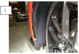
Gain access to the back side of the fog/turn signal bumper bracket. Raise the front of the vehicle using a jack and support with jack stands. Turn the wheels so that you can remove the clips holding the fender liner to the bumper.
