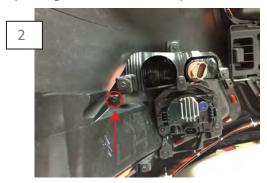
Fold back the fender liner and remove the screw circled above from the fog/turn signal bumper bracket. \*\*Note: The bumper does not need to be removed.
